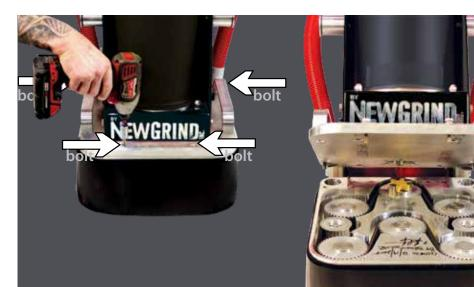
The Rhino is built with durability in mind – all machines are equipped with heavy duty extra wide drive belts for a low maintenance durable belt life. On the off chance a belt breaks, you can change it in less than 10 minutes right on your jobsite. This self-service feature is unique to our equipment, and it keeps the contractor's valuable time and money in mind.
